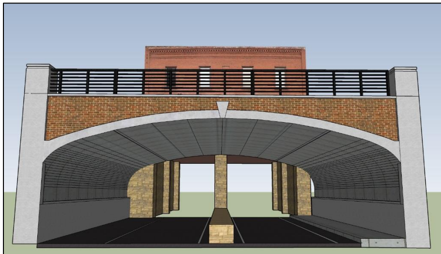
Figure 4-7: Single Span Precast Arch Option
